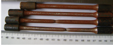
Figure 4 tensile specimen deformation diagram According to the principle of volume invariance, the actual true stress is tested:
